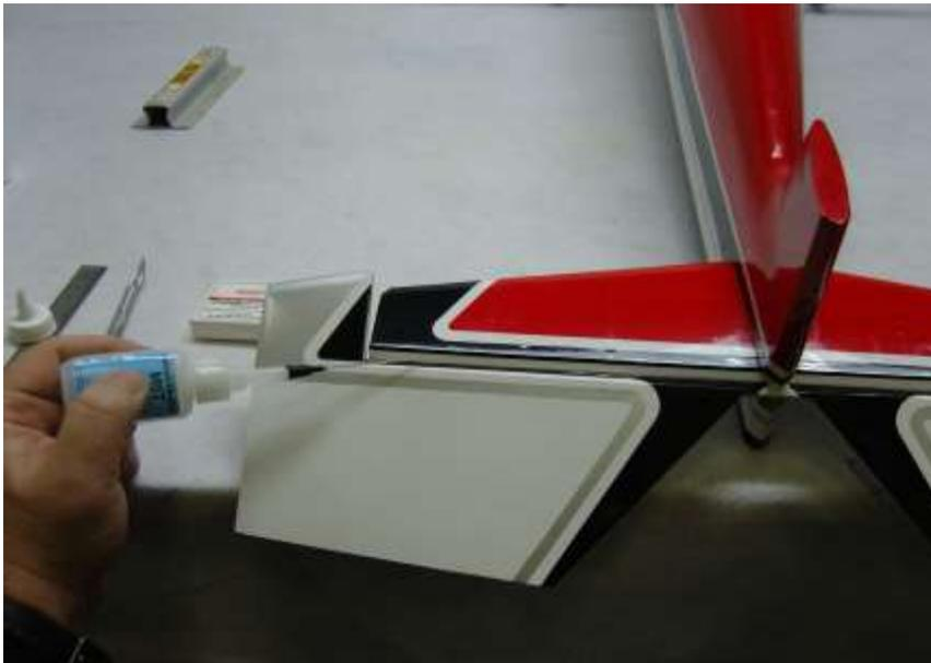
**14. Remove the covering over the slot in the lower left side of the rudder where the rudder control horn will be installed. Scuff the portion of the control horn that will glue into the surface and slide it through the baseplate. Secure the rudder control horn with medium CA.**
