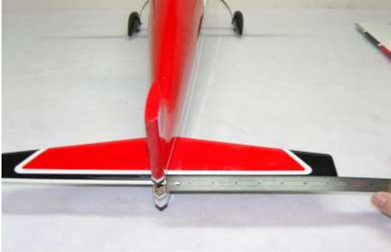
**12. Remove the covering over the left slot on the bottom of the elevator where the elevator control horn will be installed. Scuff the portion of the control horn that will insert into the elevator with sandpaper. Slide the horn into the baseplate and secure the control horn with medium CA.**
