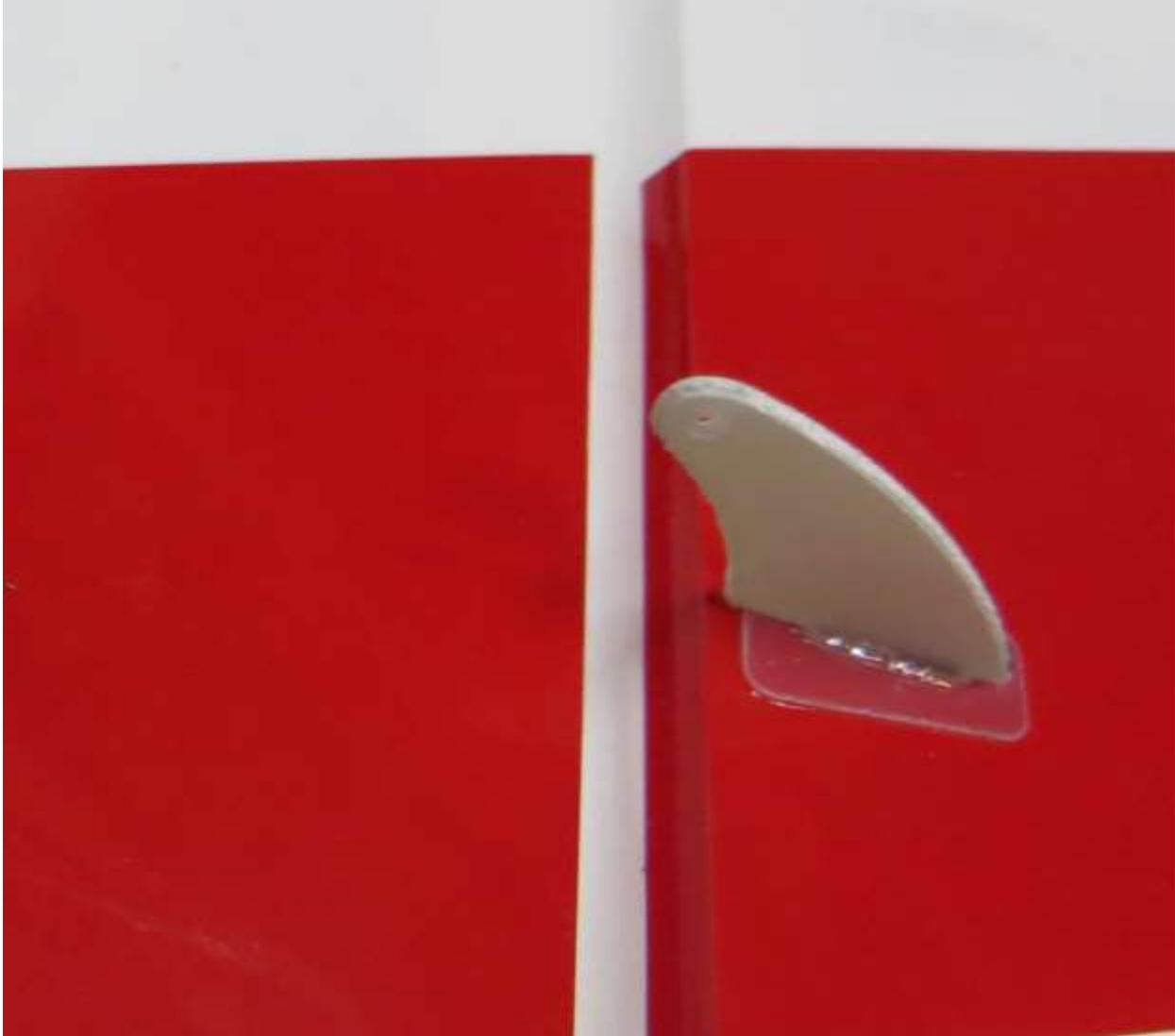
**4. Remove the covering from the aileron servo location and make sure the hinges are centered in their slots.**
