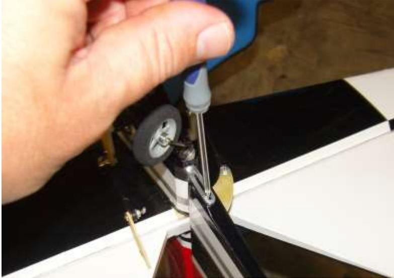
**18. Place the tailwheel wire in the proper position, aligned with the rudder and lock into place with the 2 set screws.**
