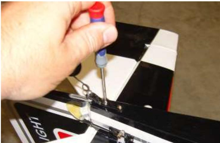
**17. Secure the tiller using the provided screw, but do not over tighten as the tiller should be able to move on the screw as the rudder is deflected.**
