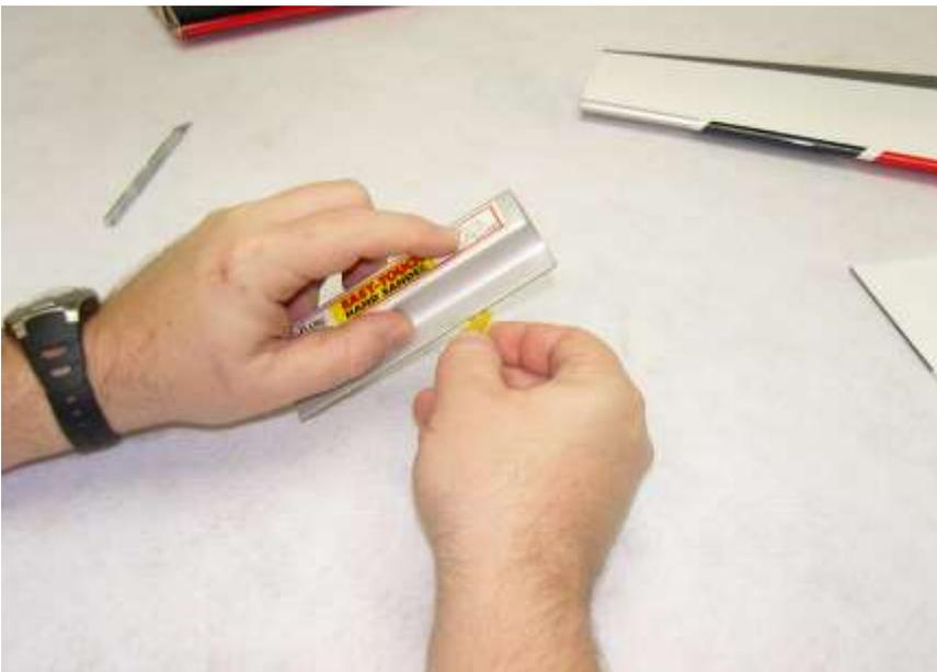
**3. Use a glue tip on your bottle of medium CA and apply glue to the slot as well as to both sides of the control horn. Insert the control horn into the baseplate and then into the slot and make sure it seats properly against the surface of the aileron. Wipe away any excess glue with a soft cloth soaked in Acetone.**
