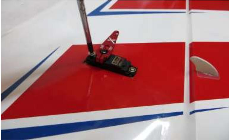
**7. Locate the 2 threaded aileron pushrods that are the same size and 4 micro ball links along with 4 2mm screws, nuts and washers. Thread the ball links onto each end of the pushrods and secure to the servo arm and control horn with the 2 mm hardware as shown in the picture. We recommend the use of the Extreme Flight lightweight electric servo arms as shown. Please note the orientation of the pushrod in relation to the control horn.**
