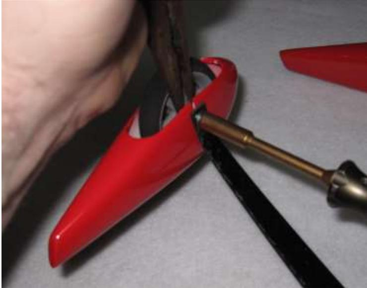
**9. Locate the fuselage, 2-3mm socket head cap bolts and 2 washers. Secure the landing gear to the fuselage by inserting a 3mm screw into a washer, through the carbon fiber gear and into the pre-installed blind nut in the fuselage. Make sure to use a drop of blue Loctite on each screw to prevent them from backing out.**
