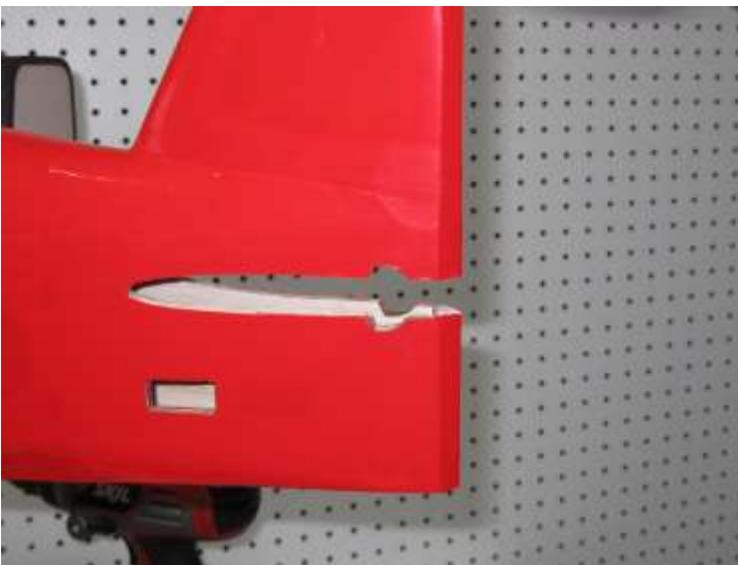
**11. Insert the stabilizer into its slot and the carbon fiber wing tube into the plastic sleeve. Use a ruler to insure that the stabilizer is centered in its slot and compare the stabilizer to the wing tube to make sure it is properly aligned. Sand or shim the slot if necessary to ensure proper alignment. Secure the stabilizer with CA.**
