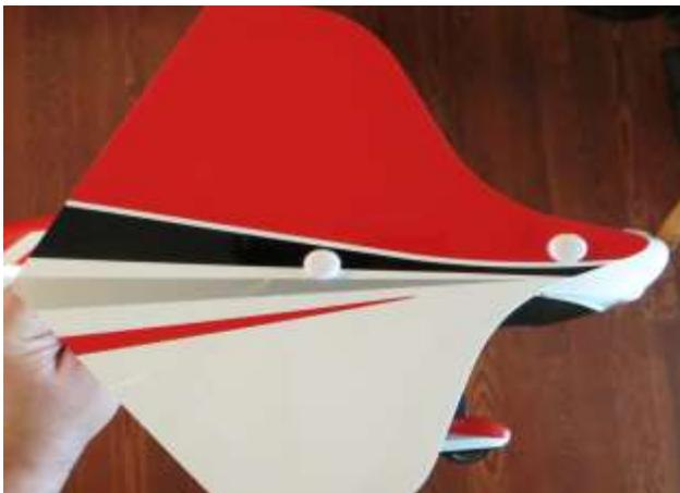
**26. Slide the carbon fiber wing tube into the fuselage and the wings onto the tube. Secure to the fuselage using the 2 3mm bolts and washers inserted through the tabs and into the pre-installed blind nuts.**
