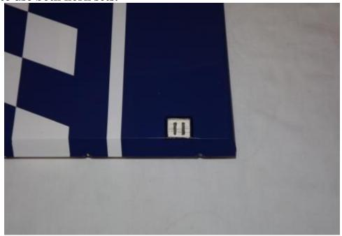
21. Mix a generous batch of epoxy and completely fill the two slots as well as the areas on the control horns and base plates that will glue into both sides of the rudder.
