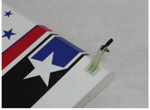
20. Trace around the baseplate with a fine tipped felt marker. Use a sharp #11 blade to remove the covering in this area for the best bond. If using the push-pull system with the rear mounted servo you will only need to glue in the horn assembly on the right side of the rudder (pilot's perspective). If using pull-pull you will need to use both horn sets.
