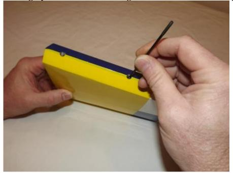
10. Next, coat one side of the hinges with epoxy and push the hinges into the holes of the horizontal stab.
