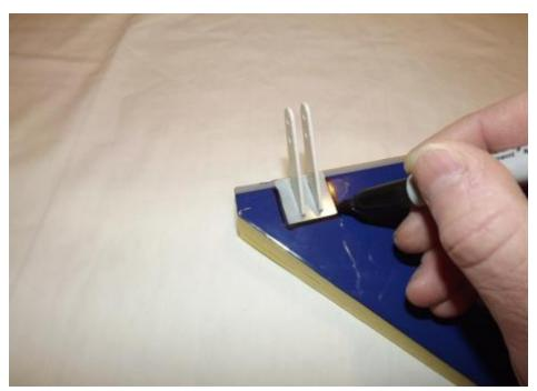
3. Remove the horn assembly and use a #11 blade to remove the covering from inside the ink line you traced around the control horn base.
