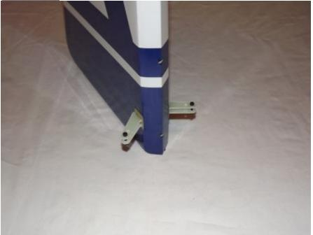
23. Locate the 2mm ball link from the tailwheel hardware bag. There is a predrilled hole to accept the shaft of the ball link. Scuff the shaft of the ball link and
