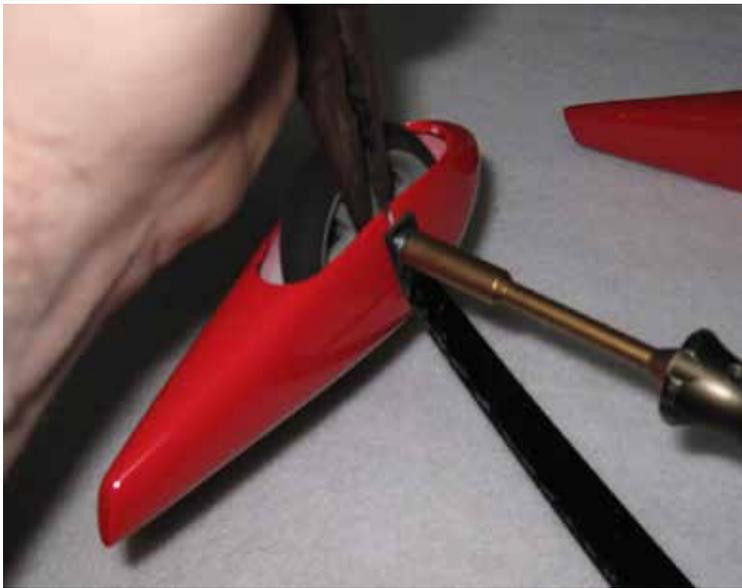
**8. Locate the fuselage, 2-3mm socket head cap bolts and 2 washers. Secure the landing gear to the fuselage by inserting a 3mm screw into a washer, through the carbon fiber gear and into the pre-installed blind nut in the fuselage. Make sure to use a drop of blue Loctite on each screw to prevent them from backing out.**
