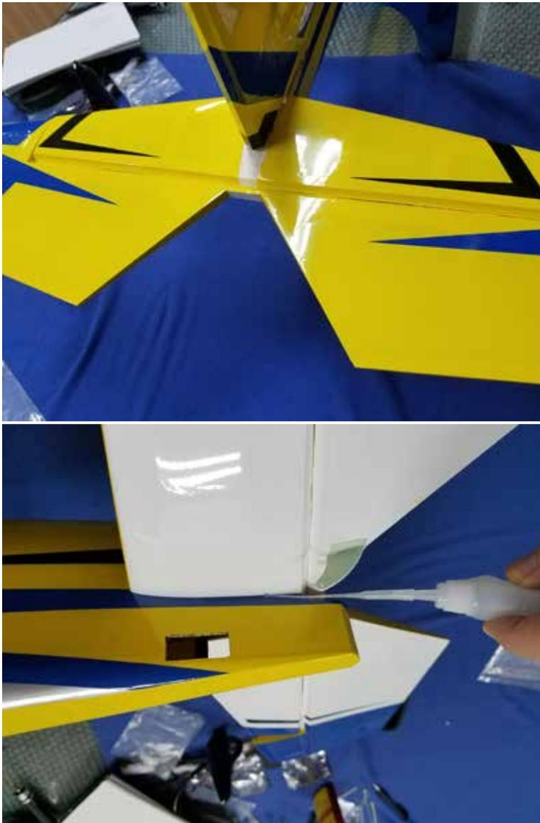
**11. Slide the elevator onto the hinges in the stabilizer and secure with thin CA. Again a fresh bottle of CA and a fine glue tip work best here.**
