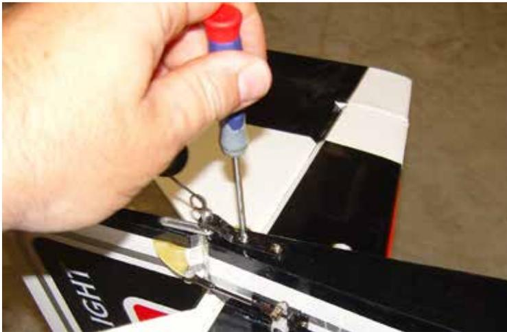
**15. Secure the tiller using the provided screw, but do not over tighten as the tiller should be able to move on the screw as the rudder is deflected.**
