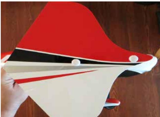
**24. Slide the carbon fiber wing tube into the fuselage and the wings onto the tube. Secure to the fuselage using the 2 3mm bolts and washers inserted through the tabs and into the pre-installed blind nuts. Plug the aileron leads into the receiver.**
