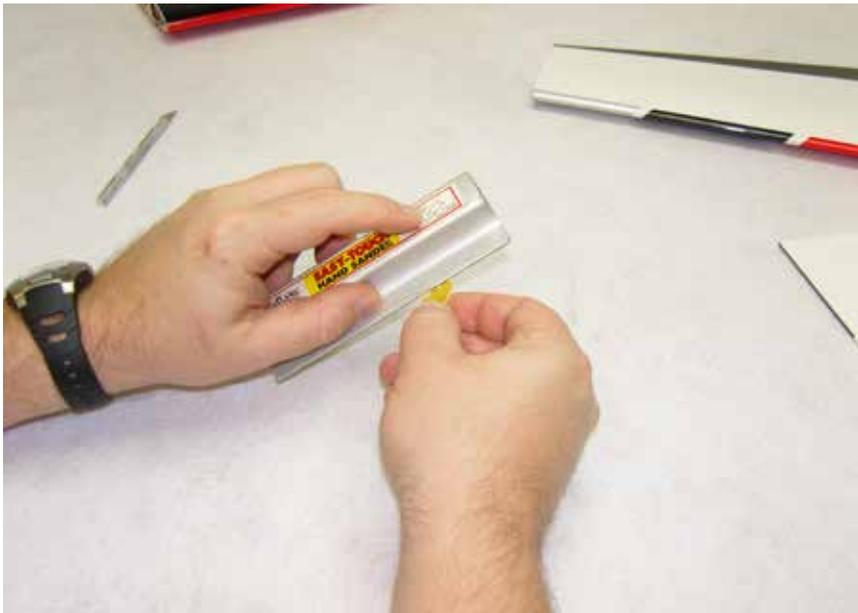
**3. Use a glue tip on your bottle of medium CA and apply glue to the slot as well as to both sides of the control horn. Insert the control horn into the**
