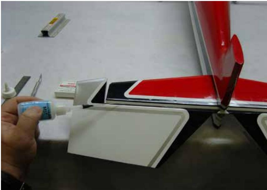
**12. Remove the covering over the slot in the lower right side of the rudder where the rudder control horn will be installed. Scuff the portion of the control horn that will glue into the surface and slide it through the baseplate. Secure the rudder control horn with medium CA.**
