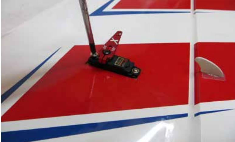
**6. Locate 2 of the threaded pushrods and 4 micro ball links along with 4 2mm screws, nuts and washers. Thread the ball links onto each end of the pushrods and secure to the servo arm and control horn with the 2 mm hardware as shown in the picture. We recommend the use of the Extreme Flight lightweight electric servo arms as shown. Please note the orientation of the pushrod in relation to the control horn.**
