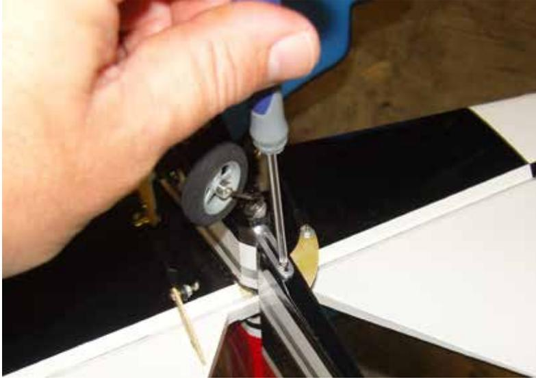
**16. Place the tailwheel wire in the proper position, aligned with the rudder and lock into place with the 2 set screws.**
