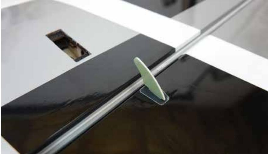
4. Slide the aileron into position on the hinges and secure with several drops of fresh thin CA. This process is much easier and more effective if a fine glue tip is used. Make sure to deflect the surface as pictured while applying the CA.
