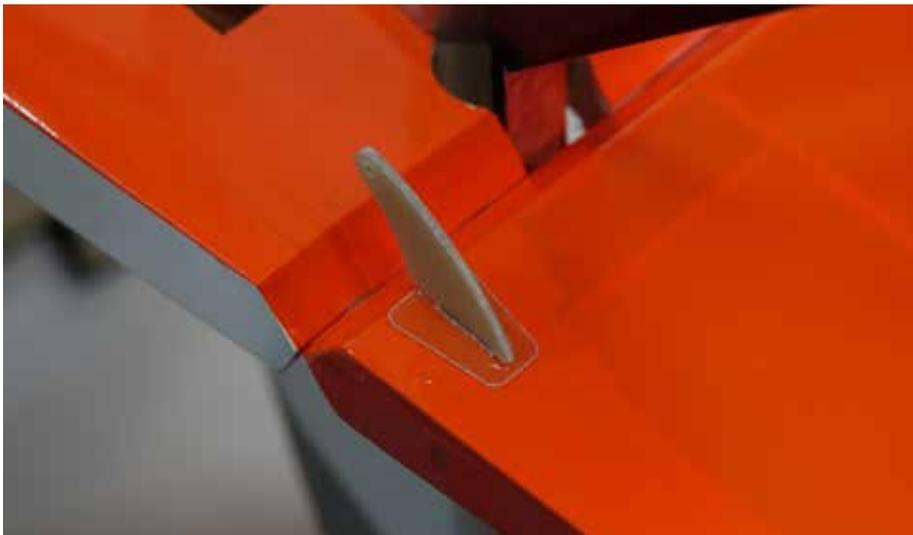
**13. Using the same process as with the ailerons and elevator, slide the rudder onto the hinges and secure to the vertical stabilizer with thin CA.**
