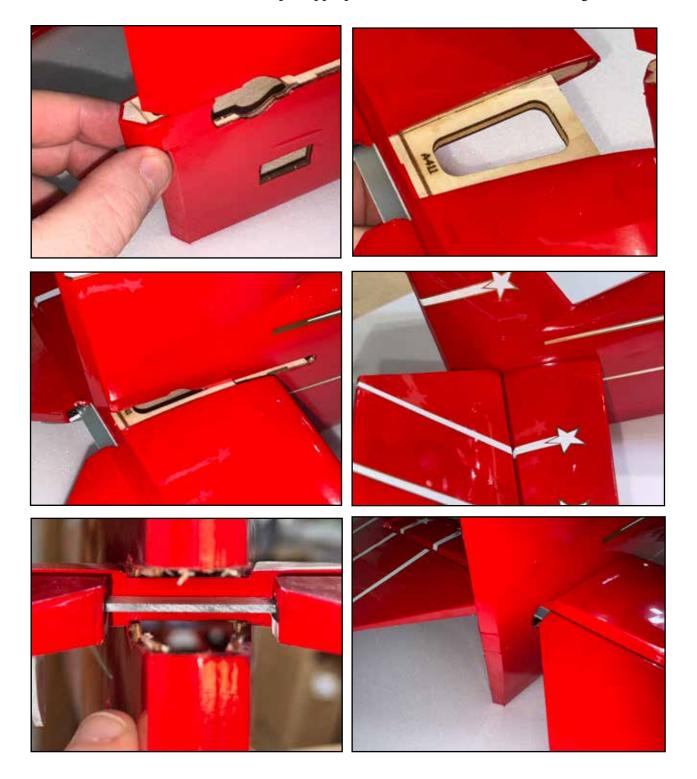
The rudder is installed by inserting the flat hinges into slots in the vertical stabilizer. Spend a little time to line everything up, once you get the hinges and slots properly lined up, the hinges will easily insert into the slots with a slight back-and-forth sawing motion.
