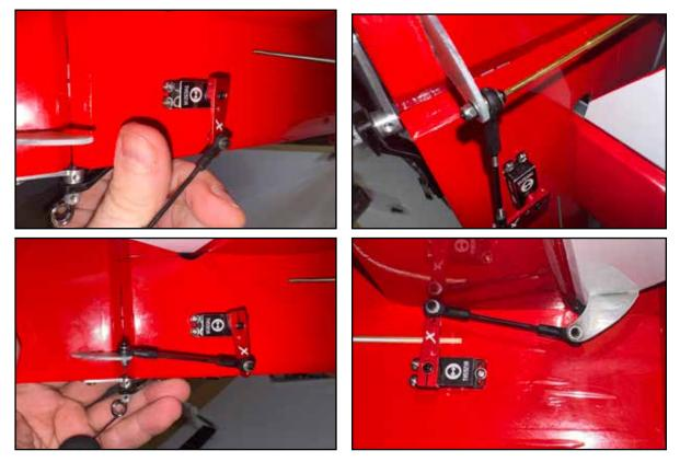
For the aileron servos, run the wires a shown, using a rubber grommer from your kit as indicated. Note that when the linkage is properly installed, it is "crooked" at the neutral position and becomes "straight" at full deflection.
