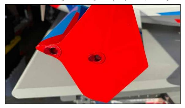
Your kit includes a cosmetic cover plate for the landing gear mount area. Install it with two dollops of rubberized glue as shown, we prefer Gorilla brand "Clear Bond" glue, Goop or Silicone are good alternatives.
