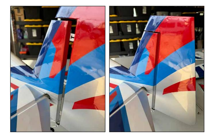
Turn the airplane on its side and apply 1-2 drops of thin CA directly onto each hinge. It will wick into the hinge slot and cure very quickly. Once the rudder is glued, replace the screw on the bottom of the rudder so it engagaes the tailwheel tiller as shown. Don't tighten fully, the tiller needs to be able to slide slightly. Flex the rudder and check for free movement.
