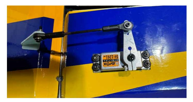
Locate the control horns for your Raven. The assembly has two parts, the horn itself, and the trim plate. Do not discard the trim plate, it holds the horn in proper position during installation. The Raven uses a pull-pull rudder assembly with two horns, one on each side of the rudder. Begin by using 120-180 grit sandpaper or emery board to scuff the horns where they insert into the surfaces as shown. This provides a good surface for gluing.
