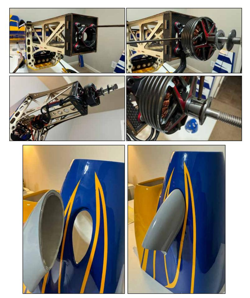
Install the clear plastic chin scoop deflector into the cowl with medium CA to deflect air toward the brushless motor. Install the cowl, spinner and prop. NOTE: Never power up your aircraft with the prop attached unless it is pointed in a safe direction and properly restrained. If you are working on your aircraft on your workbench and you need to power the system up, take the time to \*REMOVE THE PROP\* for safety.
