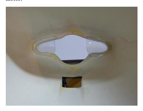
23. Slide the cowl into position and secure with 2 3mm bolts inserted through the F1 former and into the blind nuts in the cowl. A 3rd bolt is installed through the hole in the bottom of the cowl.
