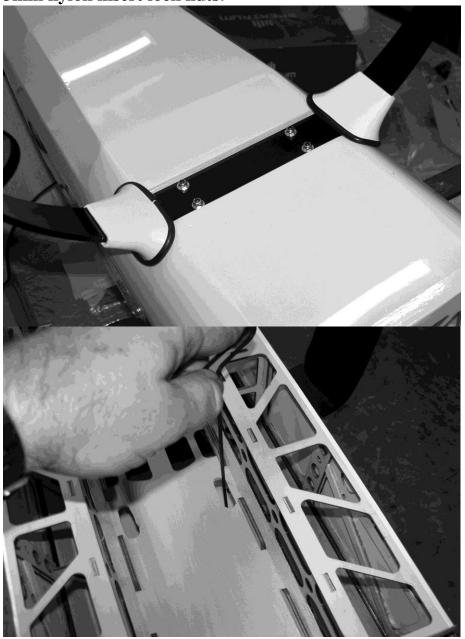
17. Locate the landing gear fairings. Slide the fairings over the landing gear and against the sides of the fuselage. You may need to open the hole in the fairing slightly with a rotary tool bit for proper fit. Use a pencil to mark the location of the bottom of the fairing on the landing gear and then remove the fairing.
