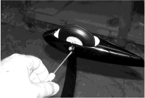
20. While the Extra is still upside down let's install the rudder and finish up the tailwheel installation. Apply 30 minute epoxy to the holes in the rudder post and to the rudder hinges. As you position the rudder onto the vertical fin, be sure the tailwheel tiller arm is inserted into the ball link. Push the rudder into position and wipe away any excess epoxy with a paper towel and denatured alcohol.
