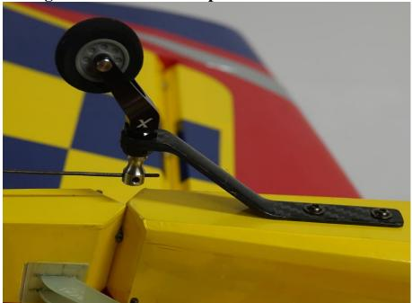
16. Next we'll install the landing gear. Locate the carbon fiber main landing gear, 4 3mm bolts, lock nuts and washers. Insert the gear into the slot on the bottom of the fuselage and center it in the slot. Secure the landing gear with 4 3mm bolts, washers and nylon insert lock nuts by inserting the bolts and washers into the pre-drilled holes in the aluminum gear mounts inside the fuselage with a long T-handle wrench. Secure with the 3mm nylon insert lock nuts.
