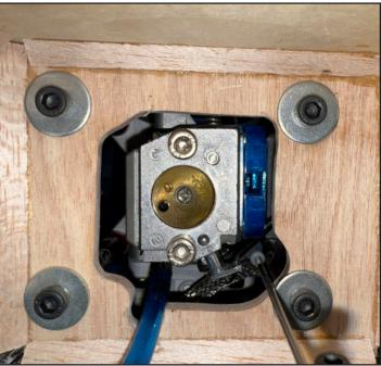
Mount the throttle servo as shown.
