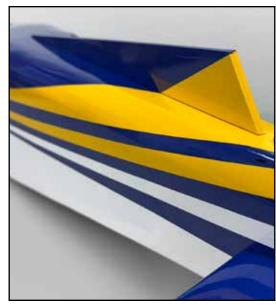
Glue the fences onto the ends of the horizontal stabilizer as shown, use CA or Goop/Gorilla Clear Grip.
