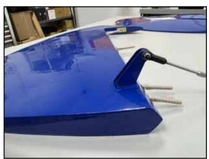
Apply good quality 15 or 30 minute epoxy into the slots and to the scuffed area of the horn. Using excess epoxy is a good idea here, as we want complete coverage and can easily clean up any excess which squeezes out with denatured alcohol on a paper towel. Press the horn firmly into the slot and make sure it seats all the way. Allow to cure.
