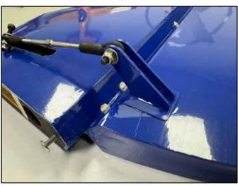
We use an epoxy gun to apply epoxy precisely into the horn slots. While the epoxy gun is a great tool, it is not necessary. If you hand mix your epoxy, be sure to get plenty of glue down into the slots.
