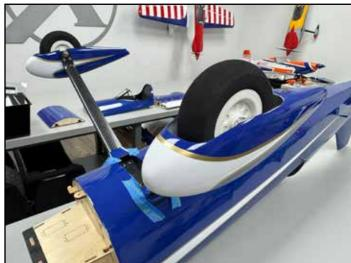
Install the tailwheel onto the fuselage with blue threadlocker. Remove the covering over the mounting hole in the bottom of the rudder and install the tiller holder (a plastic ball joint) with epoxy as shown.
