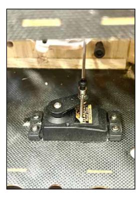
Below is the upgrade throttle pushrod. If you wish to add this to your kit yourself, the length is 135mm total, this is made from a 120mm turnbuckle and two 3mm ball links.
