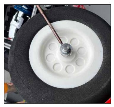
If you wish to run wheel pants, assemble and install the wheel-pant-mounts/wheel collars as shown. Two wood screws attachthe wooden wedges to the aluminum body as shown. Scuff the face of the wood wedge. Assemble onto the axle and use blue threadlocker on the set screw. Apply adhesive (we recommend Gorilla Clear Grip or Epoxy) to the face of the wheel pant mount as shown.
