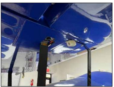
The interplane struts are retained with wire pins. At first, these pins may be very tight, requiring pliers to install/remove. If you ever need to add additional friction to these pins, we recommend a wipe of Gorilla Clear Grip glue or a little thin CA to the pin and allow to fully cure before inserting.
