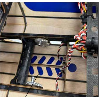
Remove covering over these vents for cooling outlet.
