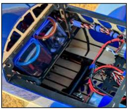
Install your fuel dot/filler as shown. For smoke, add a second dot on the opposite side. We recommend using different color dots for clarity as well, to avoid accidentally filling your fuel tank with smoke fluid. On this build, we are also using an Extreme Flight aluminum fuel vent dot on the bottom of the fuselage. Our preferred location for mounting a smoke pump is shown on the bottom of the motor box.
