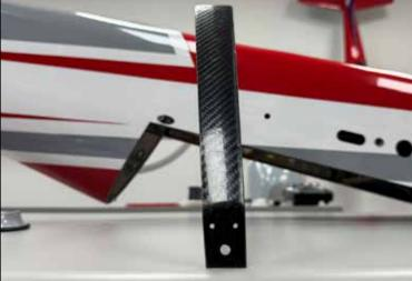
The gear attaches to the fuselage with four screws and washers as shown. Use blue threadlocker here. Install the cosmetic cover plate with ruberized glue as shown. We prefer Gorilla Clear Grip, Goop is an acceptable substitute.
