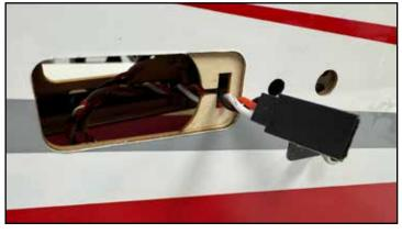
Install your rudder servo and arm. Attach the pushrod as shown, using the cone-shaped spacer on the servo-arm end of the pushrod.
