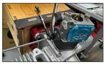
The 88" Extra 260 uses a full-size throttle servo with a 1" arm. There are two generic throttle servo locations provided, one for right-hand and one for left-hand carburetors. To get the best linkage geometry with our install, we elected to use the plywood servo mount pieces included in the kit and custom-mount the servo as shown.
