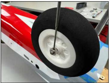
If you wish to run wheel pants, assemble and install the wheel-pant-mounts/wheel collars as shown. Two wood screws attachthe wooden wedges to the aluminum body as shown. Scuff the face of the wood wedge. Assemble onto the axle and use blue threadlocker on the set screw. Apply adhesive (we recommend Gorilla Clear Grip or Epoxy) to the face of the wheel pant mount as shown.
