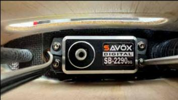
Install the servo arm, and install the pushrod, using bolts, washers, locknuts, and tapered spacers on the servo-arm end as shown. For most installations, depending on transmitter/receiver/servo type and brand, you can use the 1.75" location on the 2" arm, and maximize end points to achieve the desired throws. Maximizing endpoints and using the shortest possible arm length maximizes effective torque and resolution.
