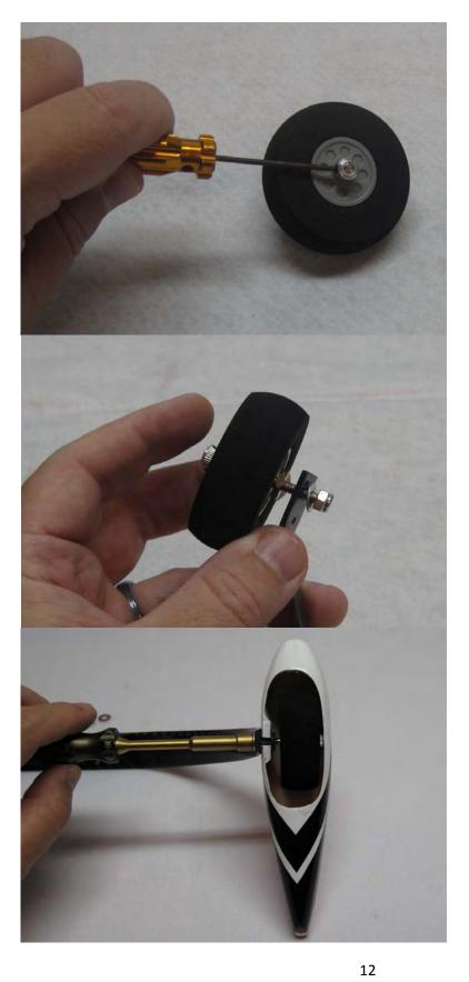
12. Secure the landing gear to the fuselage by inserting a 3mm bolt into a washer, through the carbon fiber gear and into the pre-installed blind nuts in the fuselage. Make sure to use a drop of blue Loctite on each bolt to prevent them from backing out.
