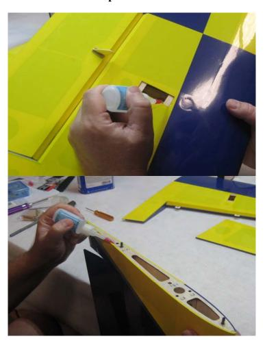
7. Use the screws provided by the servo manufacturer to secure the aileron servo in the designated location.
