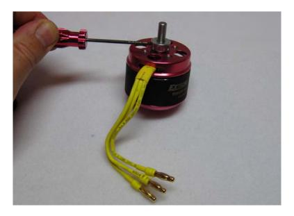
25. Next secure the radial mount to the motor using the provided short Phillip's head machine screws. Again be sure to use a drop of blue Loctite on each screw.
