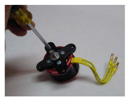
26. Secure the prop adapter using the 4 socket head cap bolts. Again blue Loctite should be applied to each bolt.
