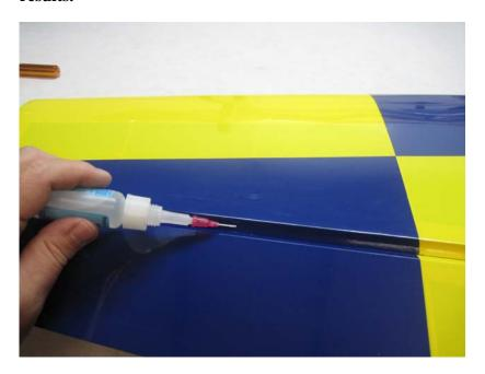
6. Before installing the aileron servo take a minute and apply some CA to the servo tray and the anti-rotation pins.
