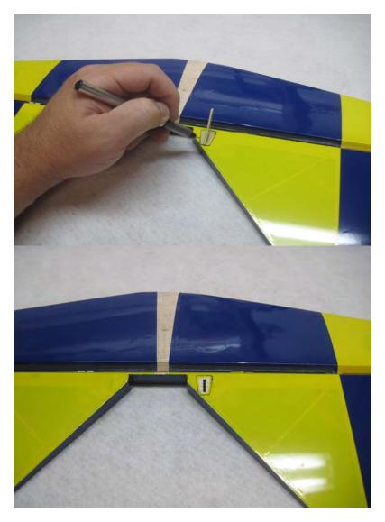
16. Slide the elevator onto the hinges in the stabilizer and secure with thin CA. Again a fresh bottle of CA and a fine glue tip work best here
