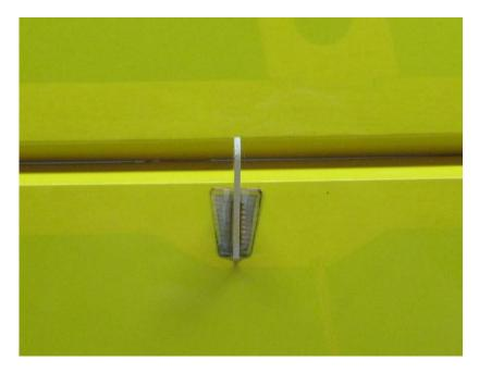
5. Remove the covering from the aileron servo location and make sure the hinges are centered in their slots. Slide the aileron into position making sure the outer tip of the aileron is flush with the wing tip. Apply a drop of CA at each hinge location on both the top and bottom side of the wing. Use a fresh bottle of thin CA and a fine glue tip for best results.
