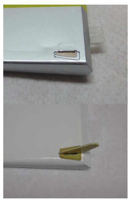
19. Using the same process as with the ailerons and elevator, slide the rudder onto the hinges and secure to the vertical stabilizer with thin CA.
