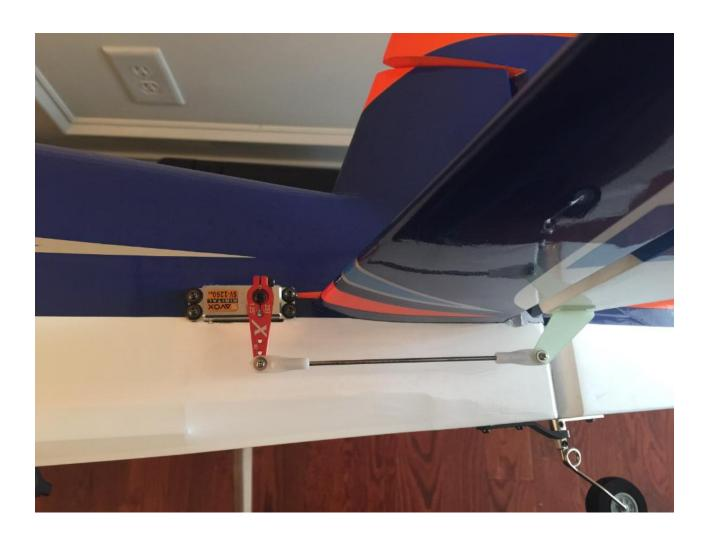
Note: Step 22 is different for the V2 60" Extra. The elevator servo is installed with the output spline towards the rear of the fuselage, as shown in the picture above.
