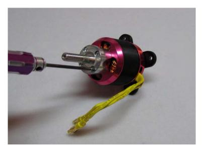
27. Mount the Torque motor using the supplied 3mm black socket head cap bolts and washers. The bolts are to be inserted into the blind nuts which are pre-installed in the motor mount plate. Be sure to put a drop of blue Loctite onto each bolt to prevent them from backing out. Be sure to add some CA to all motor box joints!
