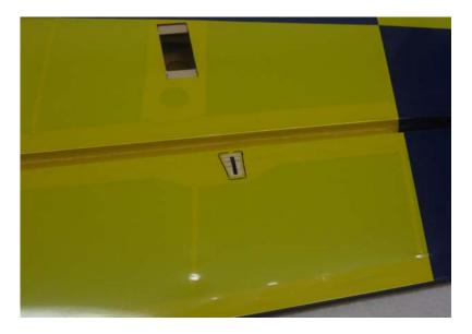
4. Mix up a batch of 30 minute epoxy and apply liberally to the slot in the aileron and to the scuffed portion of the control horn that will insert into the aileron. Install the aileron horn and base plate onto the aileron and wipe away any excess epoxy with a paper towel soaked in denatured alcohol.
