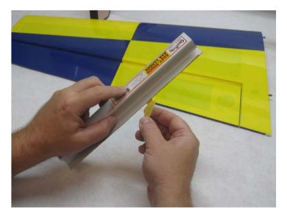
3. Use a sharp hobby blade to remove the covering 1/16 of an inch inside the line you traced around the control horn base.
