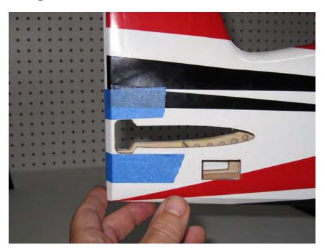
14. Use a razor saw to carefully make the cut, then sand smooth.
