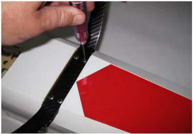
13. Next lets mount the horizontal stab. In preparation to do this we need to remove the piece of balsa at the rear of the stab slot. The factory leaves this piece intact so that the rear of the fuselage will remain true during the covering process and during transit. This is a simple process using a hobby razor saw. First place a couple strips of masking tape on the fuselage to give you a guide to cut by and to prevent the Ultracote covering from tearing.
