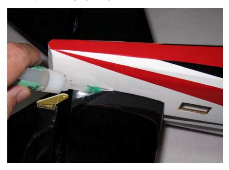
18. Remove the covering over the slot in the lower right side of the rudder where the rudder control horn will be installed as shown in the picture. <u>Use caution and only remove the covering from the lower portion so as to not penetrate the covering over the open framework.</u> Scuff the portion of the control horn that will glue into the surface and secure the rudder control horn and base plate with epoxy.
