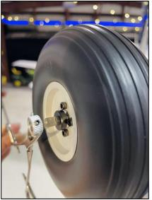
Slide on the wheels, and the wheel spacers. Note the axles have flat areas to accept the wheel collar set screws. Put blue thread locker on the set screw, then install and tighten the wheel collars using a 1.5mm hex screwdriver.
