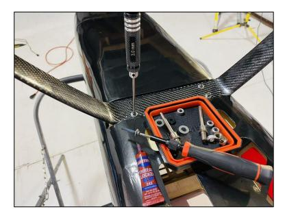
Use 4 screws and washers with blue thread locker and a 3.0mm hex screwdriver to install the landing gear as shown.
