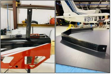
The gear has a front and a back. To identify the front, note that the gear sweeps slightly forward when installed. The best way to identify the sweep is to lay the gear on something flat.
