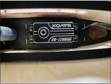
Mount the servo with a 2.0mm hex screwdriver using a drop of thin CA on all servo screws.
