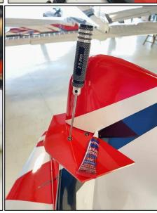
Locate the blind nuts in stabs by poking a hole through the covering then install the fins with screws and blue thread locker as shown.
