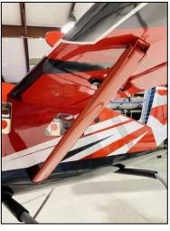
Locate the two carbon wing tubes and slide into the fuselage. Slide the wings on the tubes all the way and close the wing latches inside the fuselage. Install the struts with long screws to both fuselage and wing brackets. Once the struts are installed, then we know the strut brackets are in the correct location. Tighten the strut bracket screws fully.
