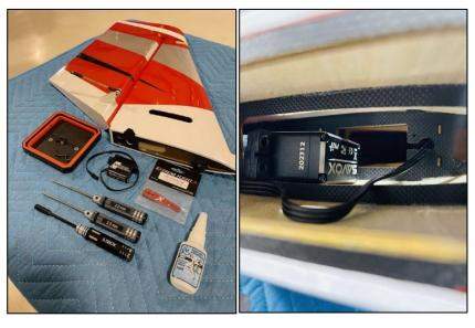
Mount your rudder servo. The servo mounts inside the vertical stab, go slowly and patiently as you place the servo into its mount. Make sure to route the servo wire through the hole. Note that the slot in the stab is placed to fit most common servos and arms, if your servo and arm combo happens to rub the wood, you can trim the slot using a hobby knife.
