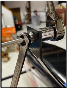
Using a 13mm socket and a 12mm wrench attach the wheel axles to the landing gear by tightening the locking nuts as shown.
